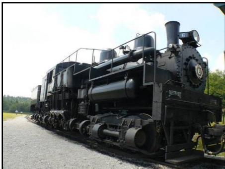
Shay engine. Note the driveshaft on the side.
